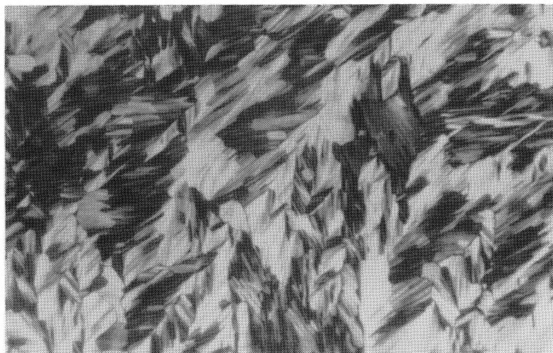
Fig. 2. Optical pattern of typical hexagonal liquid crystalline structure at 50% by weight of both water and mixed surfactant.
